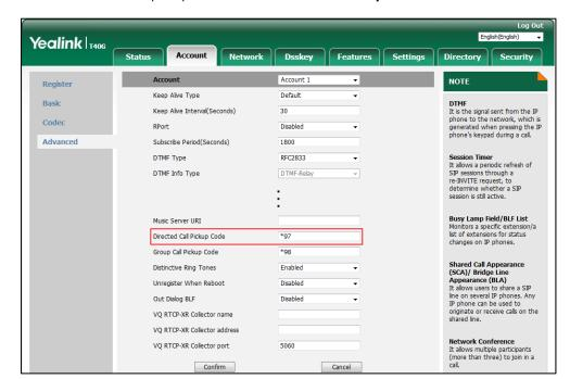
3. Enter the desired pickup code in the Directed Call Pickup Code field.
