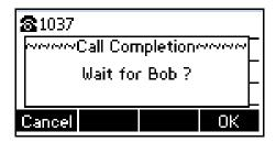
1. Press the **OK** soft key, the phone returns to the idle screen and call completion is activated.
